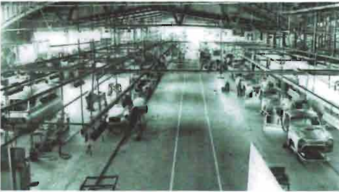
J2 vans, MGAs and Austin A50 utilities being assembled at the Enfield factory c1960
