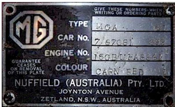
**Fig. 3.1.5 Identification Plate Type 5 (M.G. MGA 1500).**
